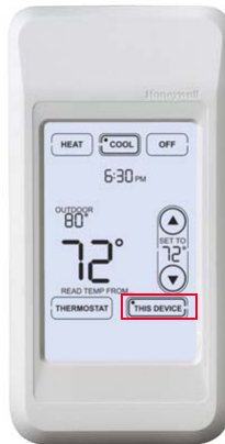
Fig. 303. Reading temperature at the Portable Comfort Control.
