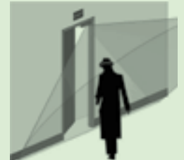
Embedded CCTV captures full facial view of persons exiting door
