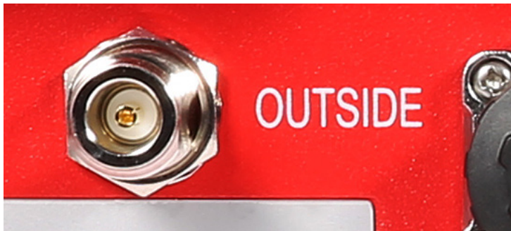
A6 — N-type Female for OUTSIDE cable and antenna
