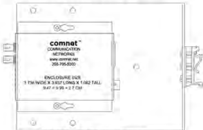
COMNET "MEDIUM SIZE" MODULE IN HORIZONTAL POSITION USE HOLES CODED "C" AND "N"
