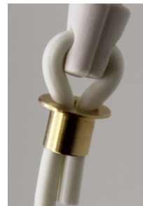
Secure the pull-cord with the eyelet, then crimp.
