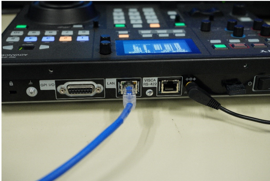
Figure 17 RM-IP500 Cabling Diagram
