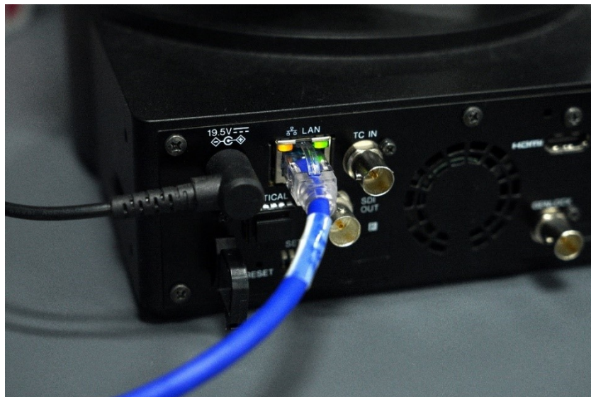
Figure 12 Cable connection diagram on the back of ILME-FR7
