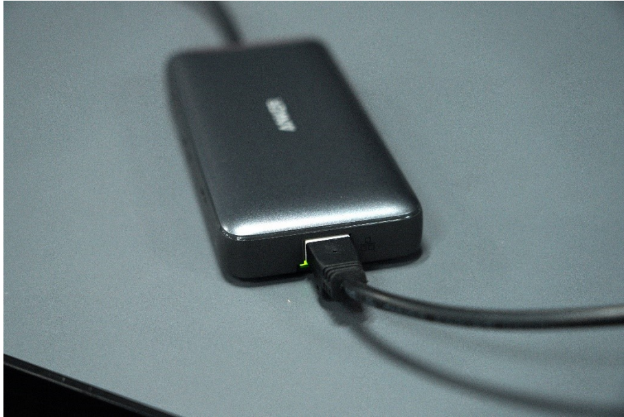
Figure 6 Connecting the LAN cable
