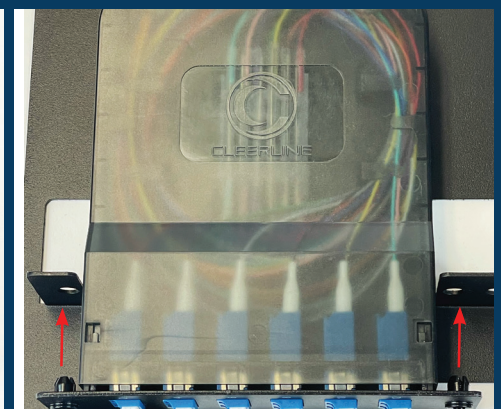
15. Locate completed cassette into any LGX sized opening, align plate so pins insert into holes, press pin plungers to lock into place completing the installation.
