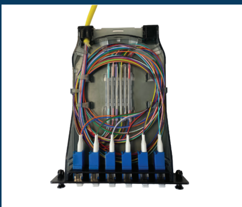
13. Check all fiber routing to ensure there are no tight bends, or fiber overhanging sides, secure if desired loosely with Velcro.
