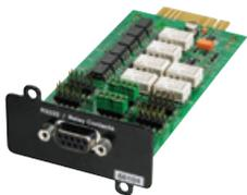
Provides communication through voltage free relays or RS-232.
