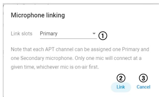
Link all microphones in the charger to the access point audio channels.
