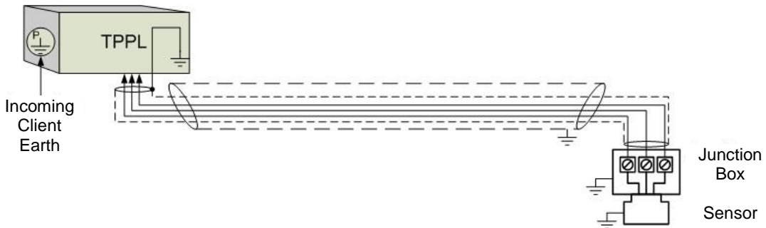
Figure 24. Grounding for Screened Cable with Armour and with Metal Junction Box and Sensor
