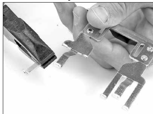
Figure 20: Prongs being broken off
