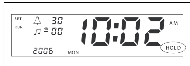
figure 6.3: Locking the controls of the front panel
