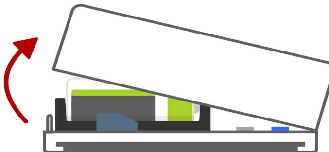
1. Use your thumb to depress the housing release tab on the bottom of the transmitter, separate the housing.
