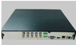
1. Loosen the screws to open the cover.
