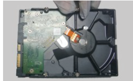
2. Screw the screws into the HDD but not tighten them.
