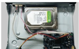
3. Place the HDD onto the bottom of the machine.
