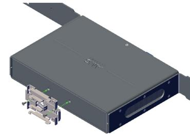
An optional DIN rail mounting kit is available. This allows for DIN rail mounting in a vertical position with the 19inch rack mount lugs removed. Fix the DIN rail clip to the AMG816 unit using the 2 x M3x6mm screws provided in the DIN rail mount kit.
