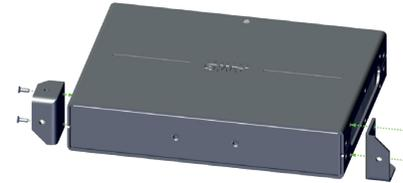
An optional wall mounting kit is available. This allows for wall mounting in multiple orientations and positions. Fix the 2 x wall brackets to the AMG816 unit using the 4 x M3x6mm screws provided in the wall mount kit.
