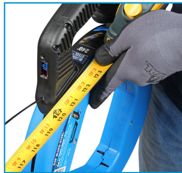
Field Calibration Press zero button Measure 10 ft. of tape Press calibration button
